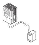
1 Connect the power wire (brown) and GND wire (blue) of the Sensor Controller's I/O cable to the 24 VDC (±10%) power supply.
